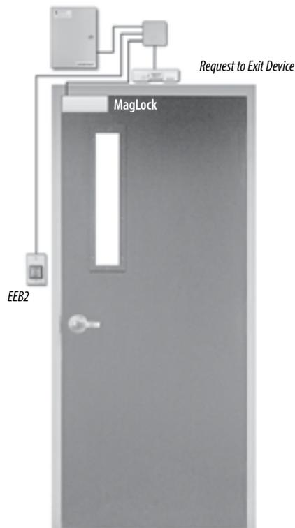
**Note:** Securitron's UL294 certification indicates that when the EEB is used with the XMS Motion Sensor, it meets the NFPA Life Safety Code 101 requirements for exit of access-controlled egress doors.
