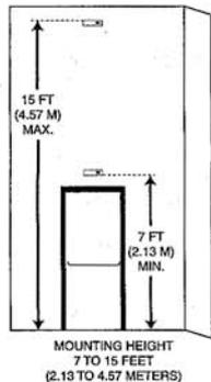
**NOTE:** If the maximum range of 8.4' (2.6m) is desired, the mounting height must be at the maximum (15' or 4.57m).
