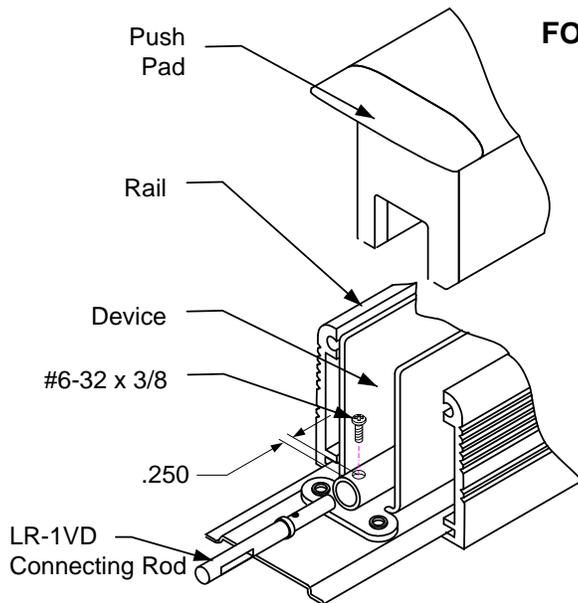
When retrofitting to existing vertical rod devices, adjustment of the rods are required for proper assembly of the LR100VDK Kit. Please see the SDC website ([www.sdcsecurity.com](http://www.sdcsecurity.com)) for installation tips and photographs of installing.
