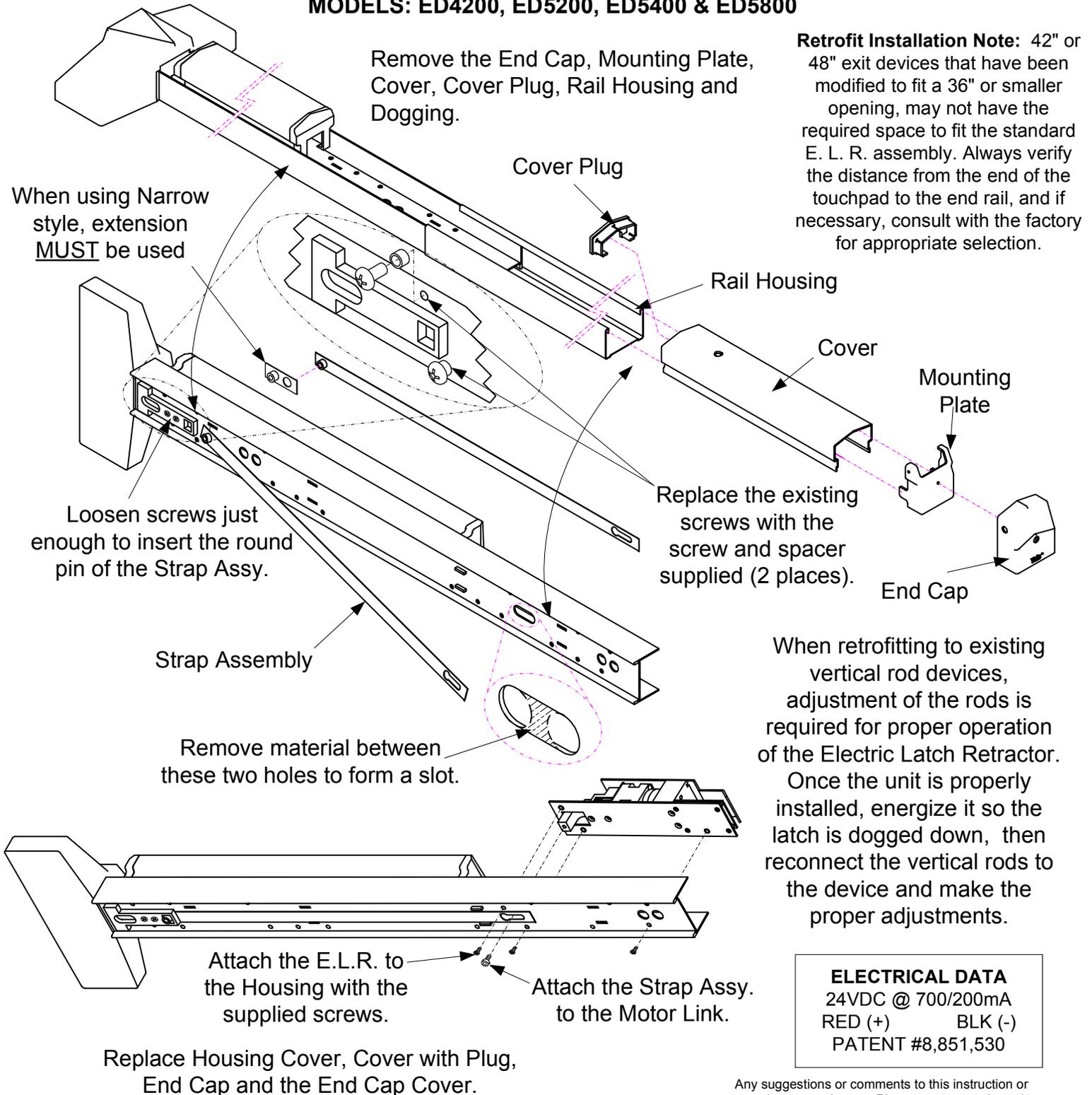
**Retrofit Installation Note:** 42" or 48" exit devices that have been modified to fit a 36" or smaller opening, may not have the required space to fit the standard E. L. R. assembly. Always verify the distance from the end of the touchpad to the end rail, and if necessary, consult with the factory for appropriate selection.
