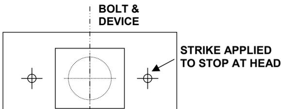
FOLD 90° ON DOTTED LINE - FOLD FIRMLY AGAINST STOP AT HEAD & INACTIVE DOOR. MARK HOLES WITH PUNCH
