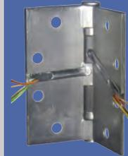
An electrified hinge must match the existing hinge. Determine the height. Determine the open width by measuring across the two leaves and knuckle when open.
