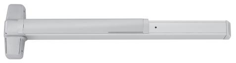
9849/9949 Concealed vertical cable device for use on single or double metal doors, UL listed for panic exit hardware. Devices are ANSI A156.3 - 2014 Grade 1. The 9849 device has a smooth mechanism case and the 9949 device has a grooved case. The concealed vertical cable device is non-handed except when the following device options are used: SD (special dogging), or SS (signal switch). See opposite page for available outside trim and device functions.
