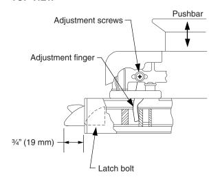
Loosen adjustment screws and adjust finger in or out until latch bolt is fully retracted (with pushbar down) and fully extended ¾" (with pushbar up).
