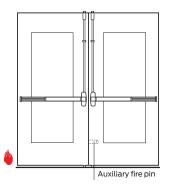
Two FEH verticle rods with auxilary fire pin-LBR option (Don't use overlapping astragal on pair swinging same direction)
