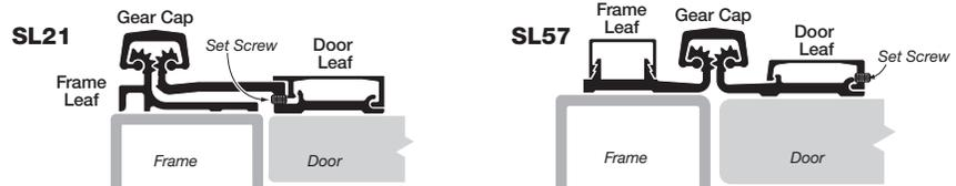
Fig. 2 Door Open Position - Leaf Covers Removed
