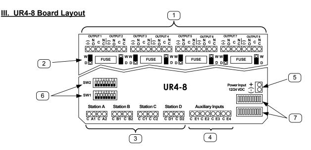
RELAY OUTPUTS – The UR4-8 provides eight (8) individual SPDT relay outputs.
