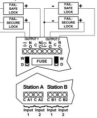
Each input may be individually configured to operate as a conventional relay or a time delayed relay. Alternatively, each input may be individually configured to operate as a latching relay or a time delayed relay.
