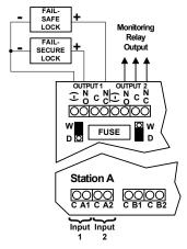
Station A Inputs activate Outputs 1 & 2 Station B Inputs activate Outputs 3 & 4 Station C Inputs activate Outputs 5 & 6 Station D Inputs activate Outputs 7 & 8
