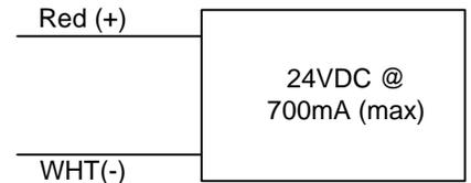
**PR1000 Input Voltage:** 12/24 VDC/VAC (+/-10%) NOTE: 1091ADMR & 1190A will operate at 24VDC only. DC voltage is recommended for optimal performance.
