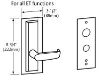
This plate is designed to be mounted behind the ET control to cover a stock hollow metal cutout
