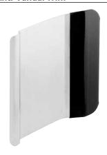
Designed for exterior doors that require extra security or resistance to vandalism, anti-vandal trim (AVT) plates have an extended lip on the active side of the door to provide extra protection for the latchbolt. A matte plastic coated grip provides a comfortable pull over wide temperature ranges. Fully through-bolted with no exposed exterior fasteners for a cleaner look and increased security.
