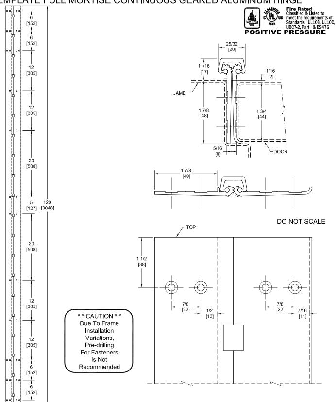
PEMKO Template Full Mortise Continuous Geared Aluminum Hinges CFM120/DFM120 are made to conform to this drawing. PEMKO CFM120/DFM120 hinges can be supplied with Electric Functions - See Electrical Application Section.
