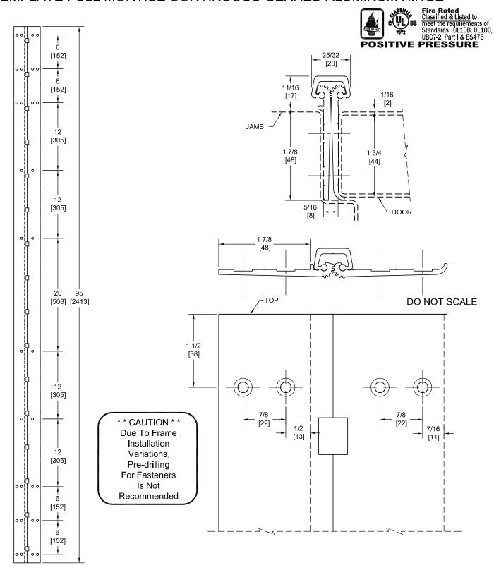
PEMKO Template Full Mortise Continuous Geared Aluminum Hinges CFM95/DFM95 are made to conform to this drawing. PEMKO CFM95/DFM95 hinges can be supplied with Electric Functions - See Electrical Application Section. Machine Screw Size - No. 12-24 x 7/16 FHUC Thread-forming.
