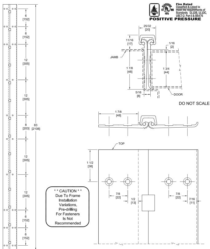
PEMKO Template Full Mortise Continuous Geared Aluminum Hinges CFM83/DFM83 are made to conform to this drawing. PEMKO CFM83/DFM83 hinges can be supplied with Electric Functions - See Electrical Application Section. Machine Screw Size - No. 12-24 x 7/16 FHUC Thread-forming.
