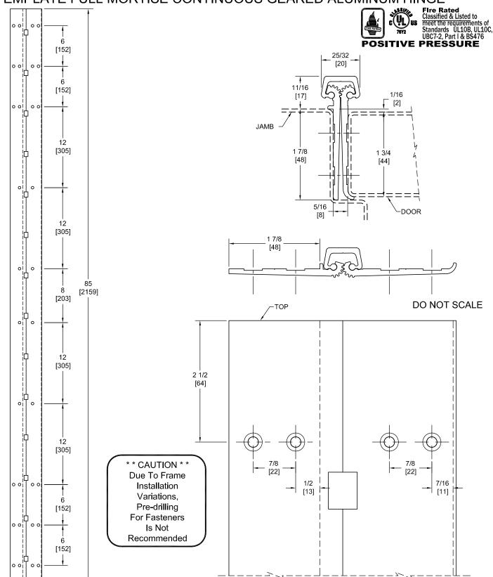
PEMKO Template Full Mortise Continuous Geared Aluminum Hinges CFM85/DFM85 are made to conform to this drawing. PEMKO CFM85/DFM85 hinges can be supplied with Electric Functions - See Electrical Application Section.
