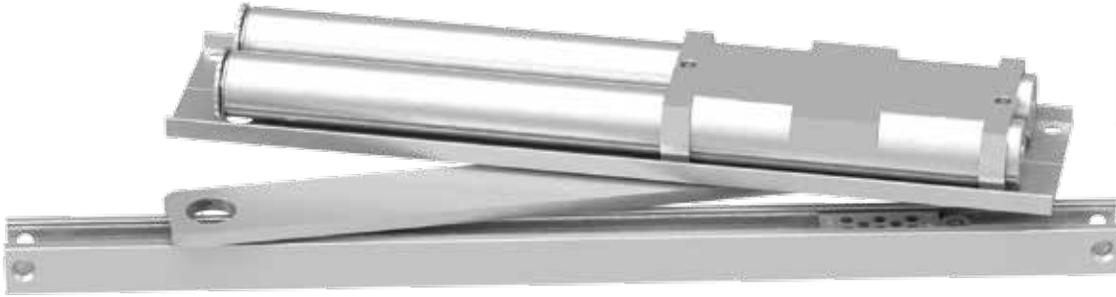
The concealed 6030 Series PACER® is a heavy duty, double acting closer designed to fit in a narrow, minimum 1-3/4" header. The single lever arm and roller assembly provides smooth, quiet door control and the choice of finishes and track functions meet virtually all architectural requirements. Installation at left illustrated with center pivot set (not included).
