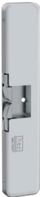
The 9400 series is a slim-line, surface mounted electric strike designed to accommodate rim exit devices with a 1/2" throw Pullman latchbolt. All components are completely encased within its 1/2" thick stainless steel housing, so no cutting on the frame is required for installation. Simply place the electric strike on the surface of the frame, align it with the exit latchbolt, and install.
