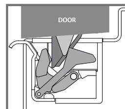
As the door moves forward, the latchbolt slides first along the keeper and then up the internal ramp.
