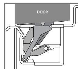
When the electric strike is energized, the keeper begins to rotate and the deadlatch platform falls away, allowing the deadlatch to drop and the latchbolt to become unguarded.
