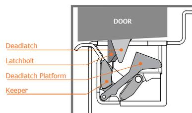
As the door continues along its arc away from the frame, the latchbolt and deadlatch exit the 8500, which quickly returns to its locked state.
