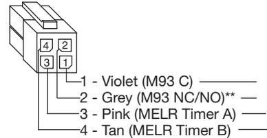
\*\* M93 NO/NC (Normally Open/Normally Closed) is selectable on controller. Factory preset is NO. Please consult SECTION IV if NC is preferred.
