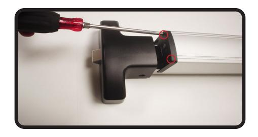
2. Slide push pad pin out of REAR activating bracket & set aside. Install REX switch with switch arm facing down. Re-install push pad pin.
