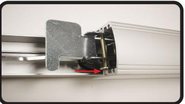
4. Slide over the FRONT activating bracket ensuring the pin & bracket is in the correct bottom channel.
