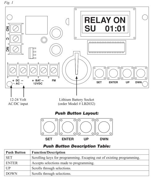
**UP** and **DOWN** keys can be used to select data entries. After scrolling to the correct entry, depress **ENTER** to accept.
