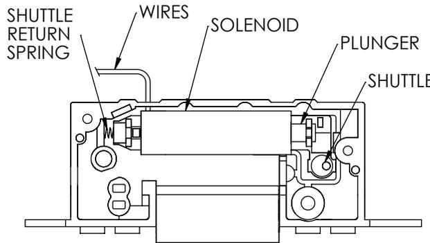
REVERSE SOLENOID AND REPLACE, ENSURING CORRECT PLACEMENT AND ALIGNMENT. WITH THE SOLENOID SEATED PROPERLY THE SHUTTLE SHOULD MOVE FREELY.
