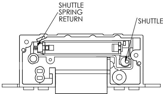
TRANSFER SHUTTLE RETURN SPRING TO OPPOSITE END OF SHUTTLE. NOTE: WHATEVER THE FUNCTION, THE SHUTTLE RETURN SPRING SHOULD ALWAYS BE AT OPPOSITE END TO THE SOLENOID PLUNGER.
