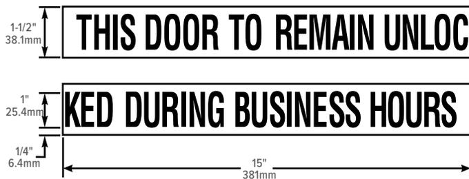
\*This sign correct under Uniform Building Code. Also includes NFPA wording "This Door to remain unlocked when the building is occupied".
