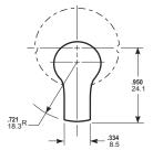
**Dimensions of Cam to Operate:**
